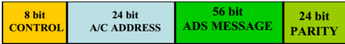
Figure 4.2 Extended (112 bit) squitter
