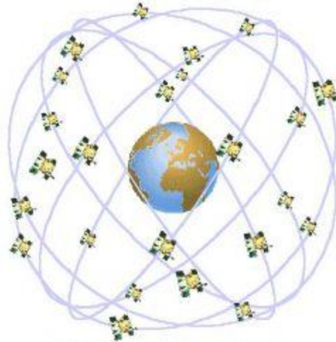
GPS Nominal Constellation: 24 satellites in 6 orbital planes, 4 satellites in each plane, 20,200 km altitude, 55 degree inclinations
