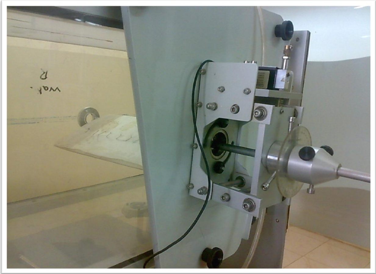
Figure 5-10: explain the angle adjustment device
