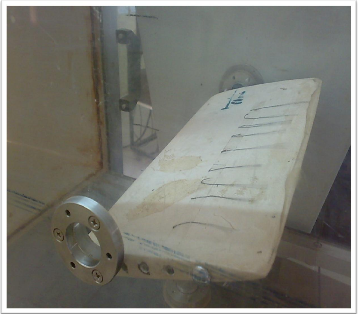
Figure 5-11: the load in position (13) and influence of air to the filaments at certain angle.
