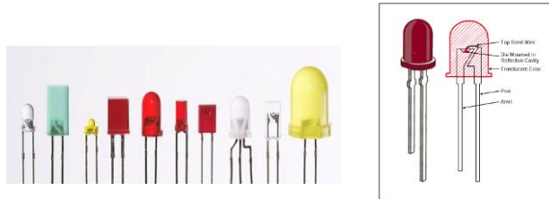
Figure 3.7: LEDs types' actual photo and internal structure
