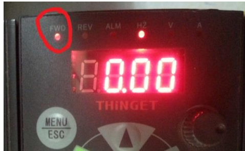
Figure 4.7: FWD indicator in screen inverter
