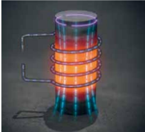
Figure 2.1 flows of eddy currents in the work piece
