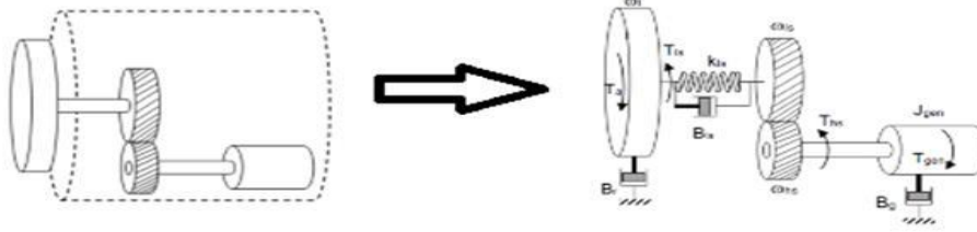
Figure (3.4): Typical gear of wind turbine
