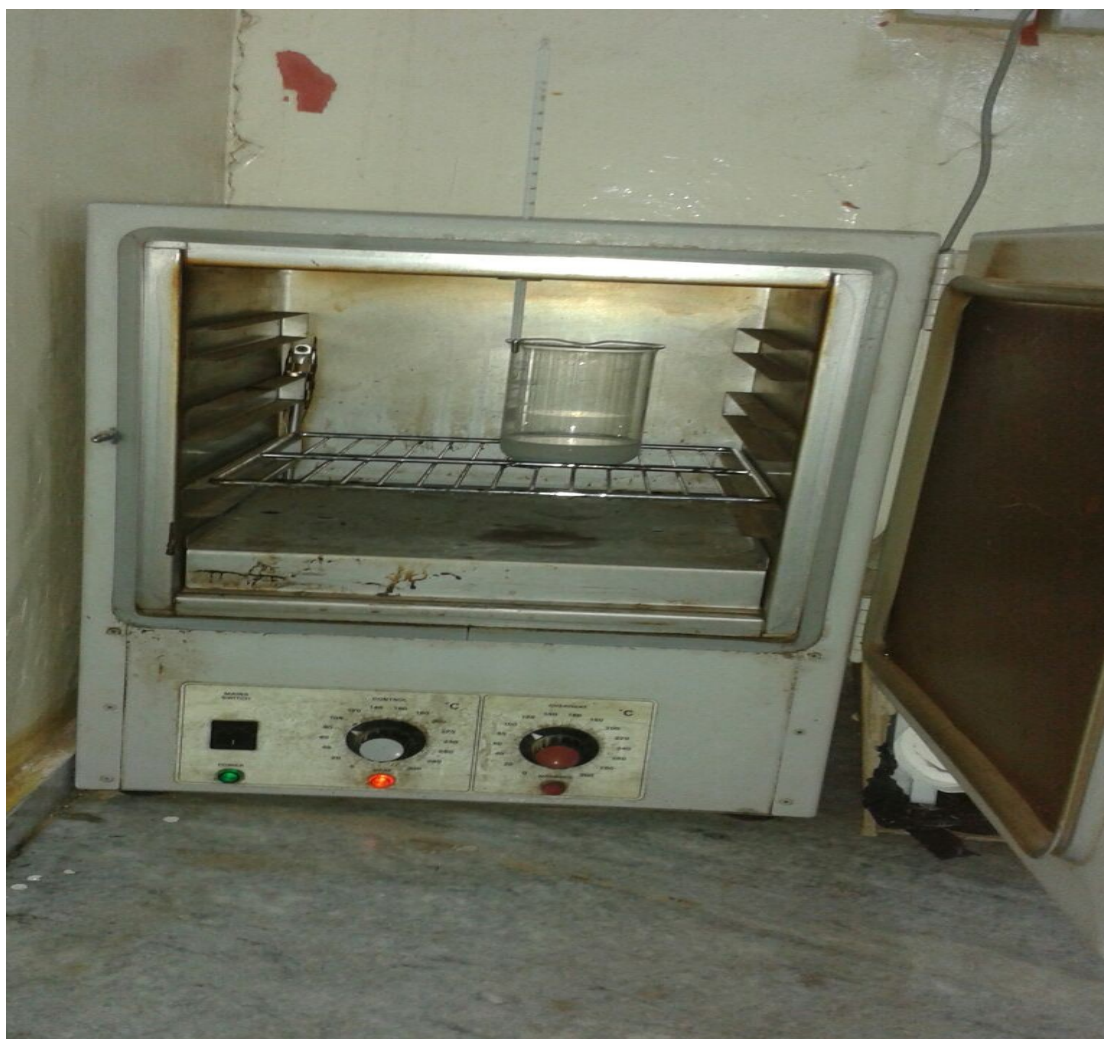
Figur 3.3 solution inside an oven heated at temperature 90^{\circ}\text{C} for 3 hours solution .
