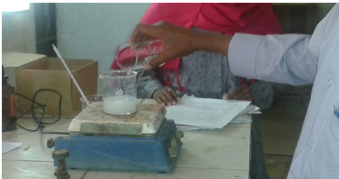
Figur 3.1 heat the solution to 60°C under continuous stirring
