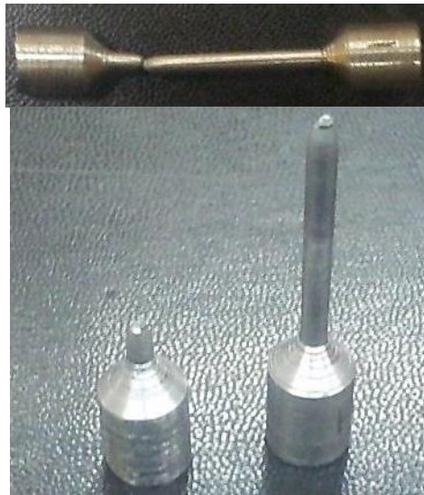
Figure 4.3 Fracture of tensile specimen tested at room temperature
