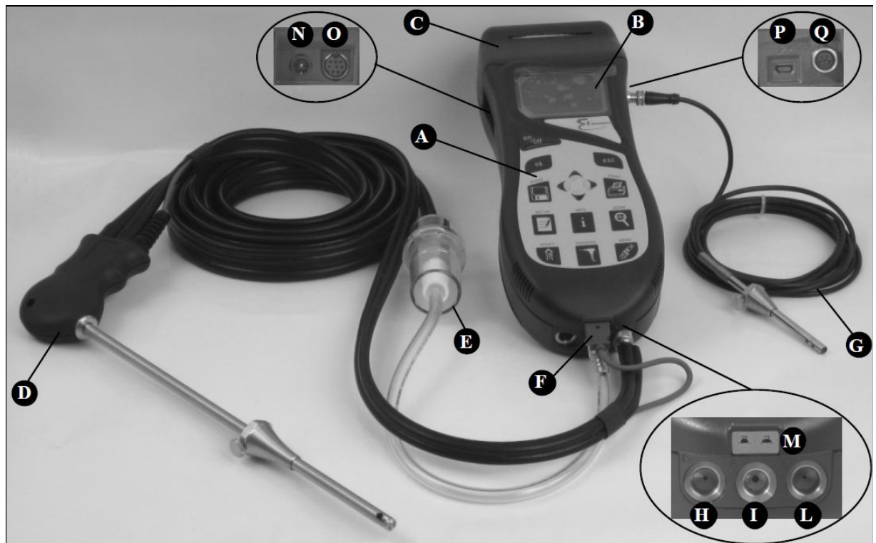
Fig (4.2) Overview of Flue Portable Gas Analyzer Components
