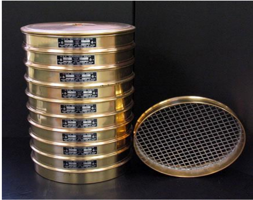
Figure 3-2: Stacked Sieves used for A gradation and Size Test
