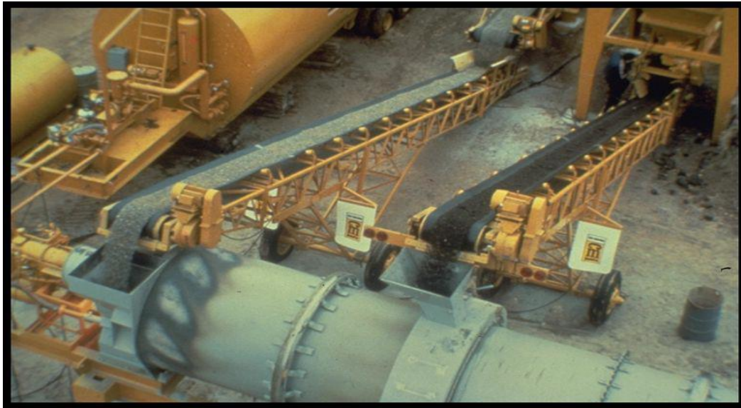
Figure 3-9: Introduction of RAP Material in A drum Plant.
