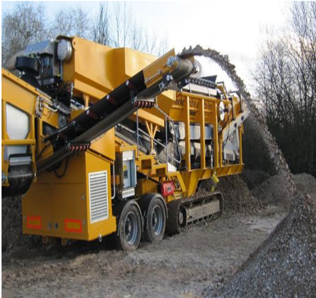
Figure 3-17: Star Screen and Mixing Machine in Soil Stabilization
