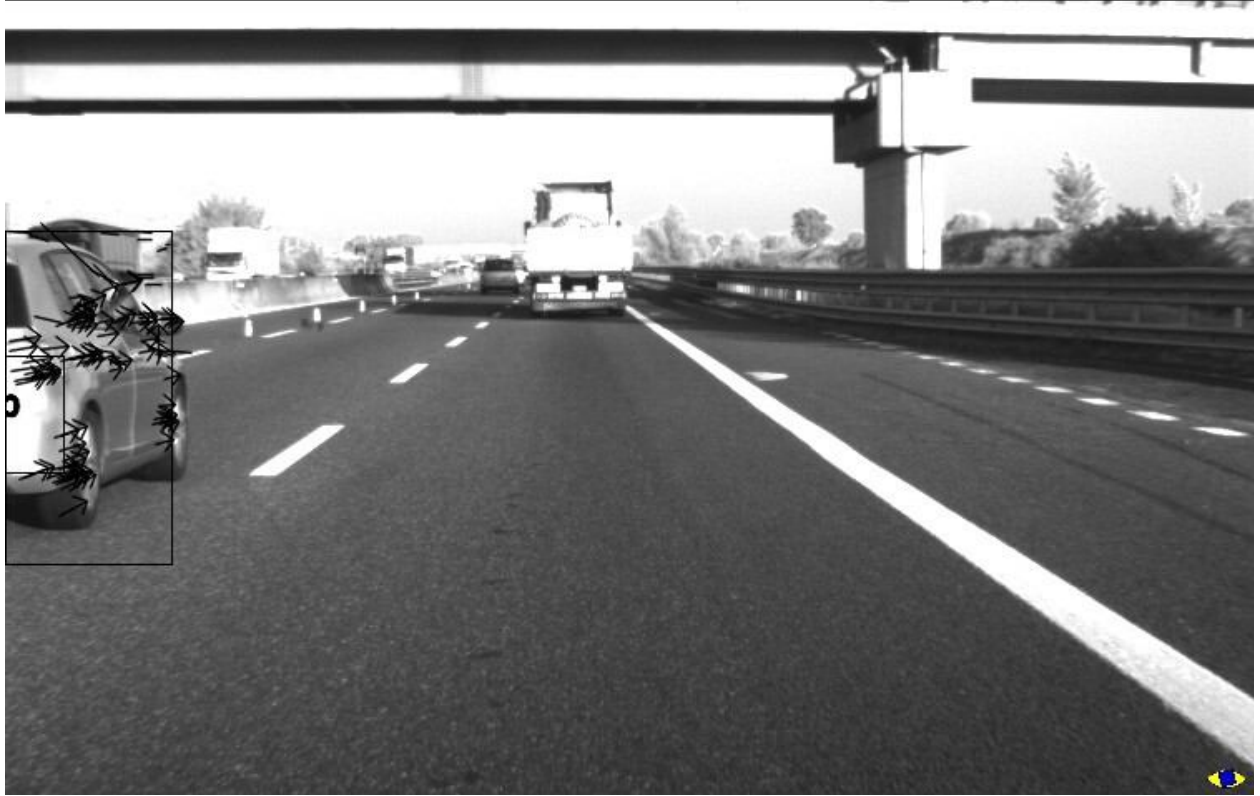
Figure 3.7: Radar detection of a vehicle outside the field of view of the camera and optical flow positive detection.
