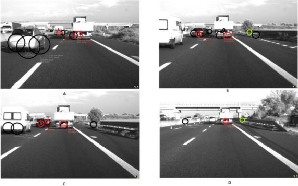
Figure3.6: Raw radar data detections on black, vehicles detection given by the ECU on red, and not moving detections on green. A Multiple detections for a single vehicle. B Misdetetection of an overtaking car. C and D not vehicles detections at laterals.
