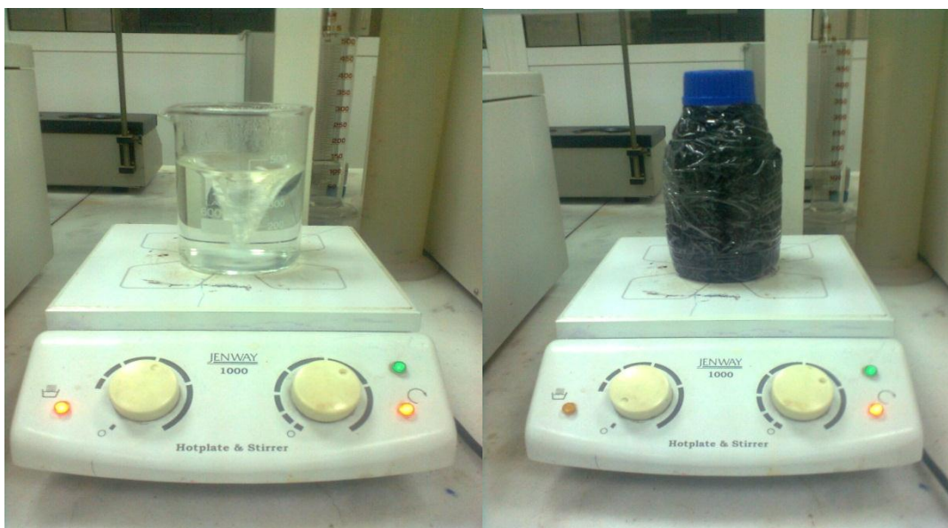
Figure 3.7 shown the dissolving PVA/AgNo 3 in distilled water using magnetic stirrer and hotplate
