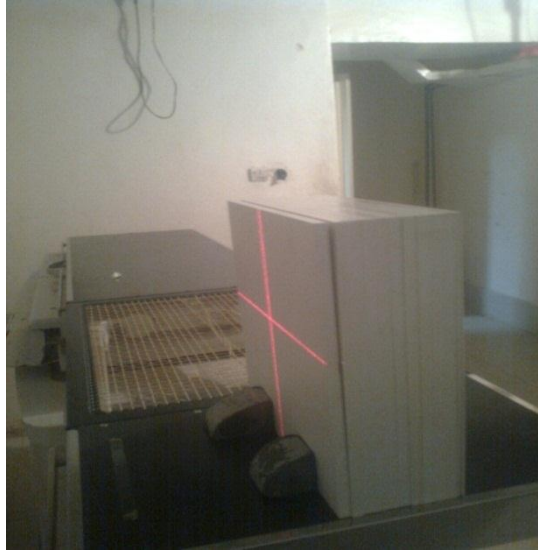
Figure 3.8 shown the films position during irradiation by ^{60}\text{Co} teletherapy machine.
