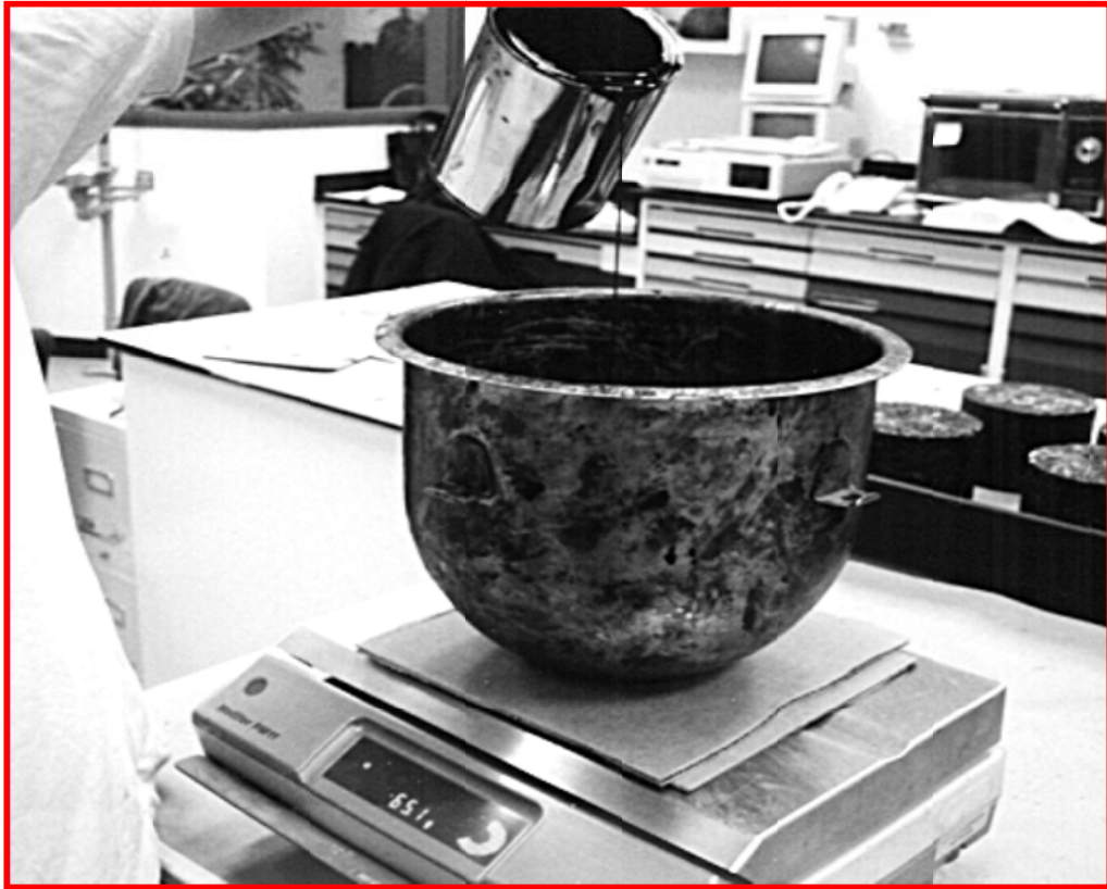
FIGURE 3-2 Added the required asphalt weight to the aggregate in the mixing bowl
