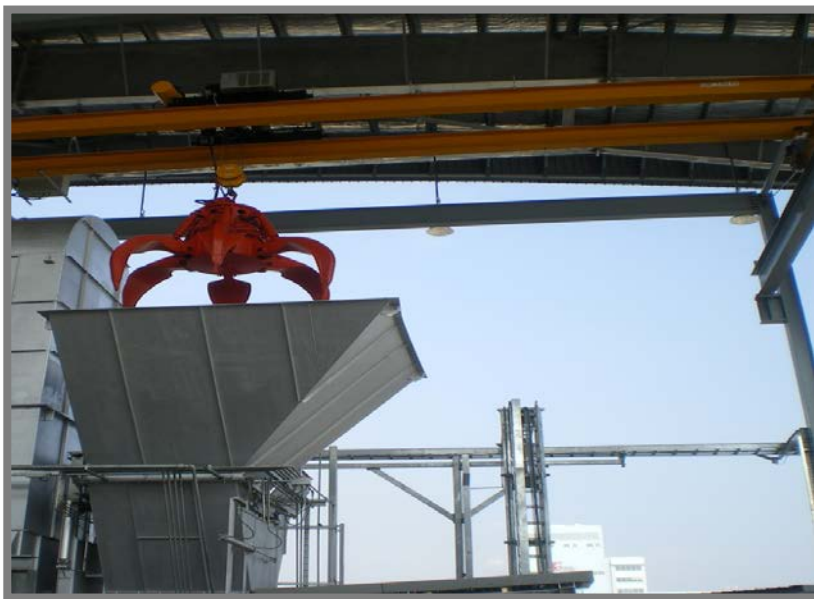
Figure (5.19b) Waste feeding system using Grip crane
