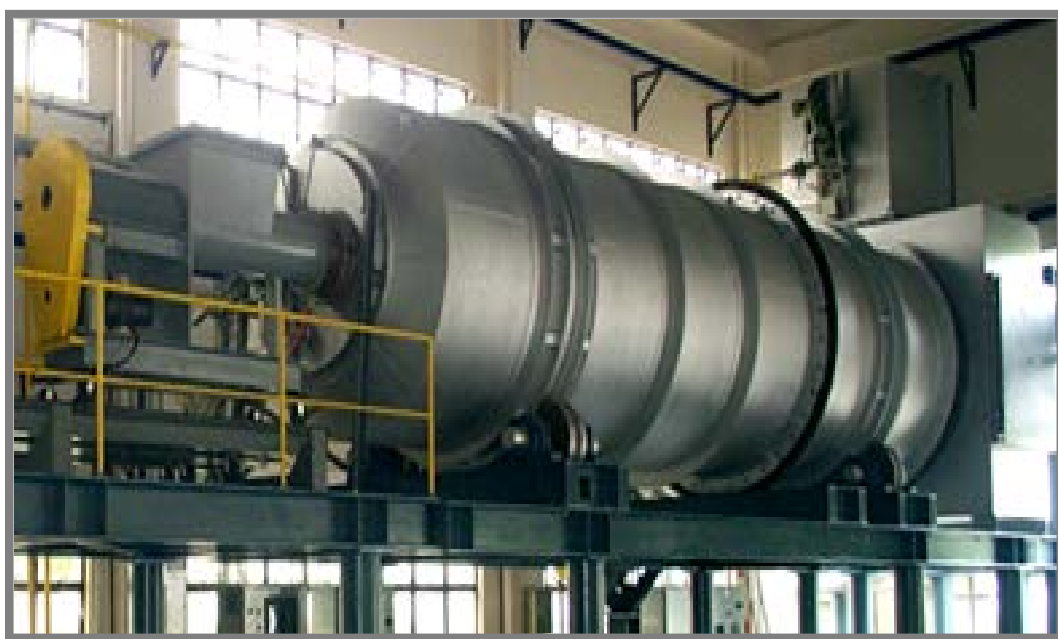
Figure (5.20d) Rotary shell with feeder and burner
