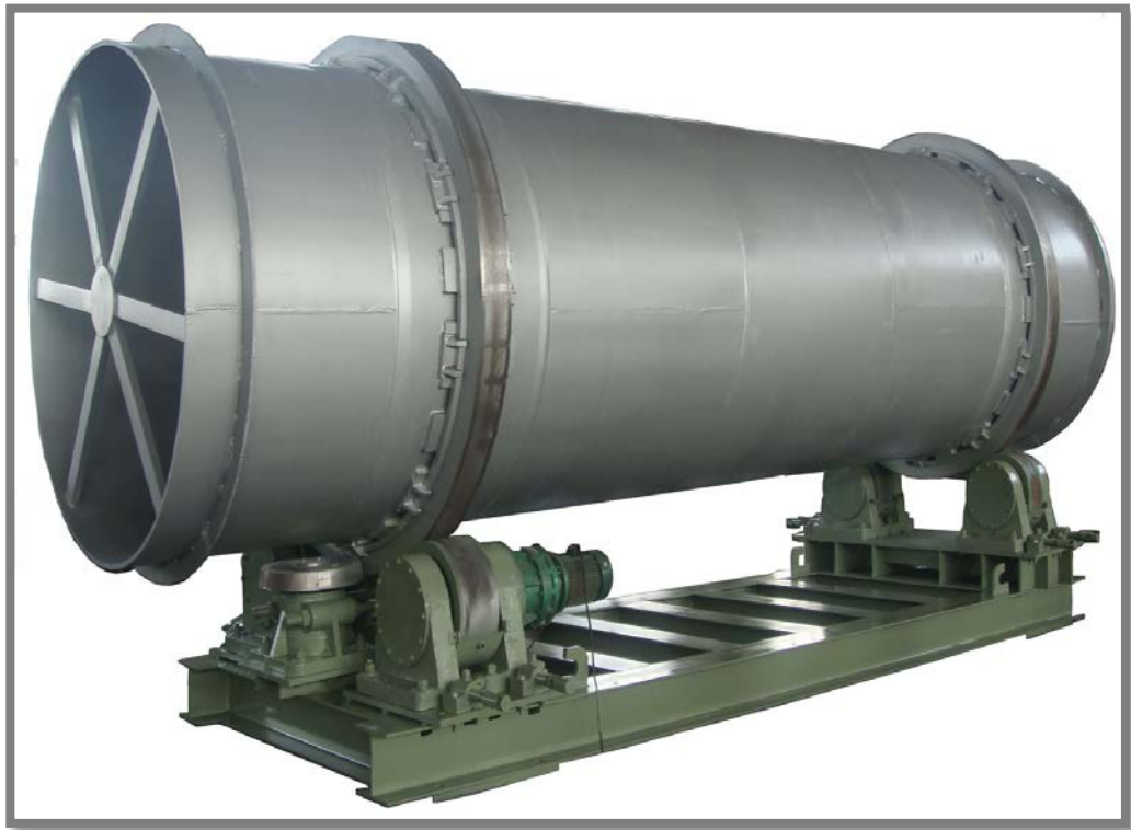
Figure (5.20b) Rotary shell with Tyres and rollers
