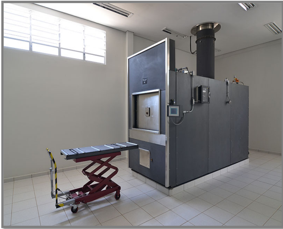
Figure (5.16a) Excess air incinerator
