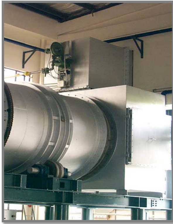
Figure (5.40) Rotary kiln burner attachment
