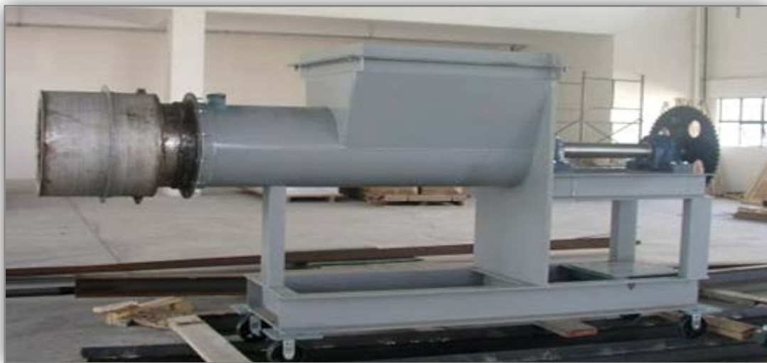
Figure (5.18c) High temperature injection screw conveyor
