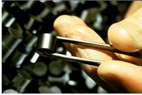
Figure (3.1) : A nuclear fuel pellet
