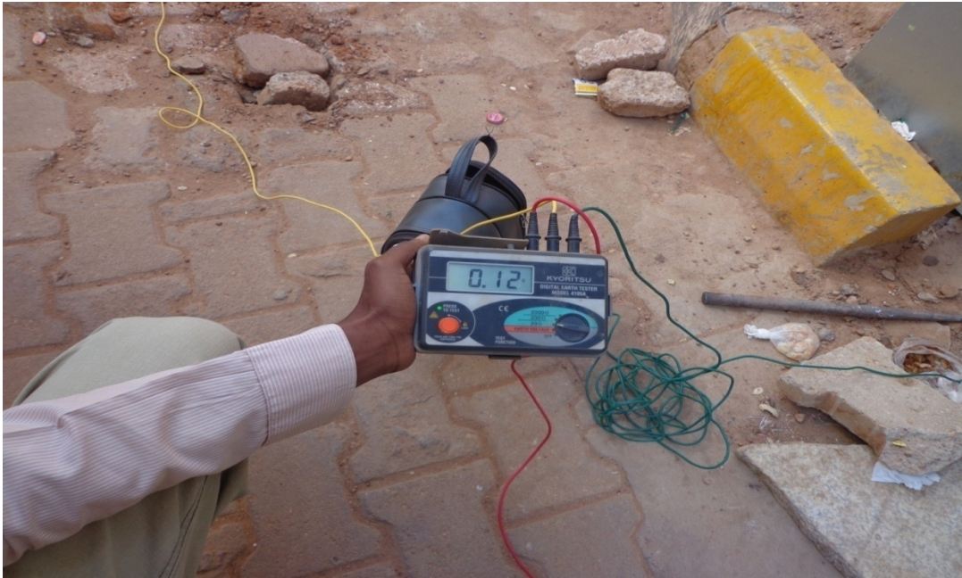
Figure 5.8: image showed the resistance earth read using digital earth tester in the fifth case.
