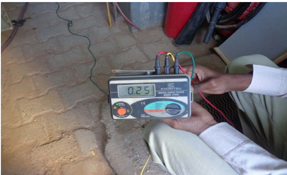
Figure 5.9: the image showed another reading for earth resistance from another point using digital earth tester.
