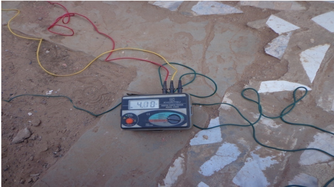
Figure 5.10: the image showed the earthing resistance read which was taken using digital earth tester in the seventh case.
