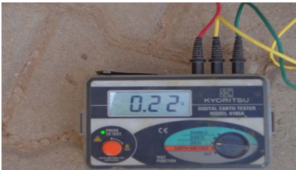
Figure 5.3: image showed reading of the check point after baring part of the main grounding cable using digital earth tester. One of the poles of the device has been connected with the grounding rod system, and the second is connected to a rod of steel was installed inside the ground just 5 meters from the ground rod, and the
