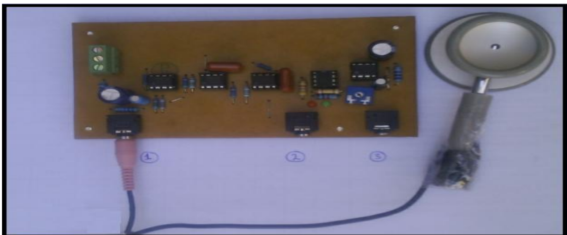
Figure (3.10): shows the integrated PCB circuit of an electronic stethoscope.
