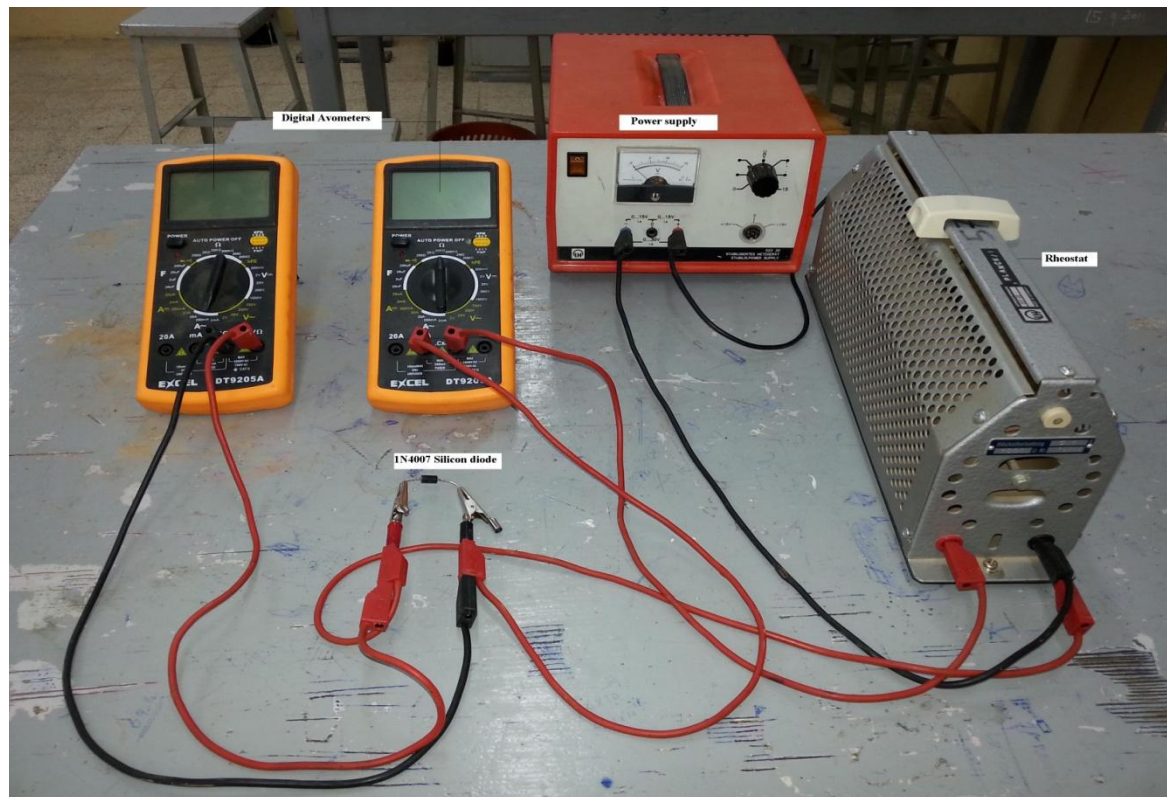
Figure 3.5 Setup for I-V measurements for pre irradiated 1N4007 silicon diode
