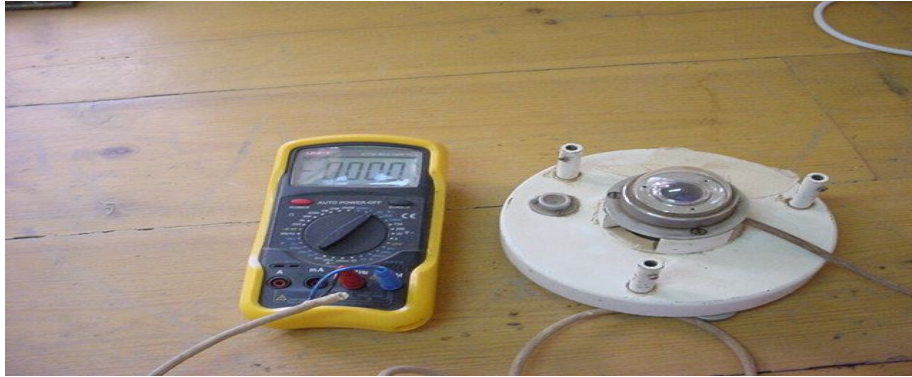
Fig.3-2. solarimeters and digital Multimeters
