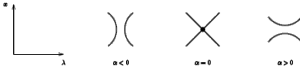
Figure 6.1 Solution diagrams for f(x, \lambda, \alpha) = x^2 - \lambda^2 + \alpha = 0 . The transcritical bifurcation point is destroyed for \alpha \neq 0
