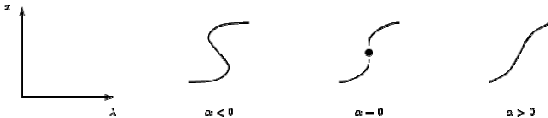
Fig. 6. 2. Solution diagrams for f(x, \lambda, \alpha) = x^3 + \alpha x - \lambda = 0 . The hysteresis point is destroyed for \alpha = 0 and there are no singular points for \alpha > 0
