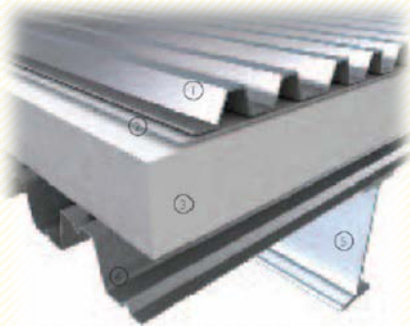
1-D detail view of rib profiled metal sheet roof
