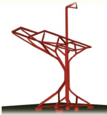
Tree Column Steel Structure
