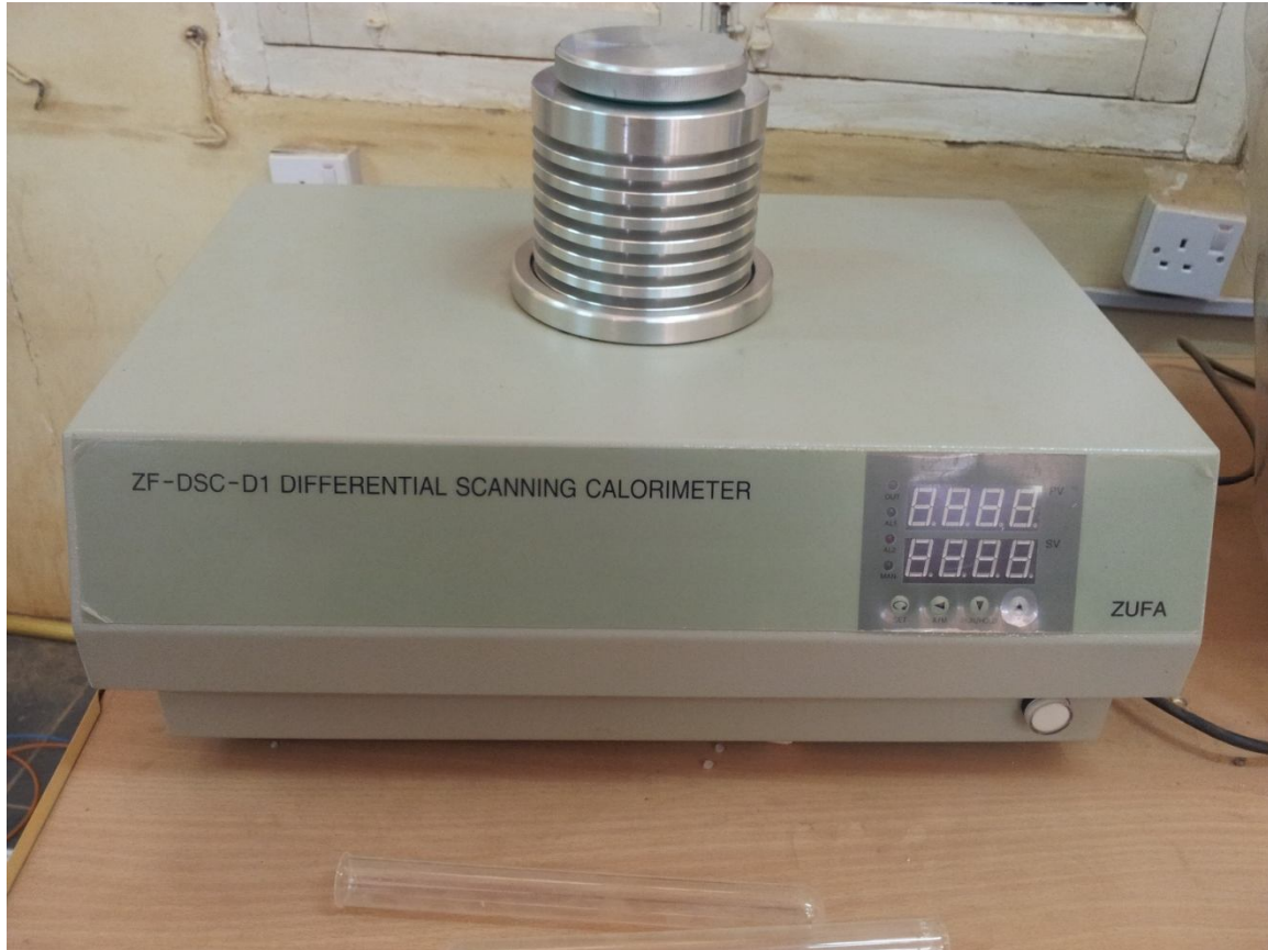
Figure 3.2 : ZF-DSC-D1 Differential scanning calorimeter
