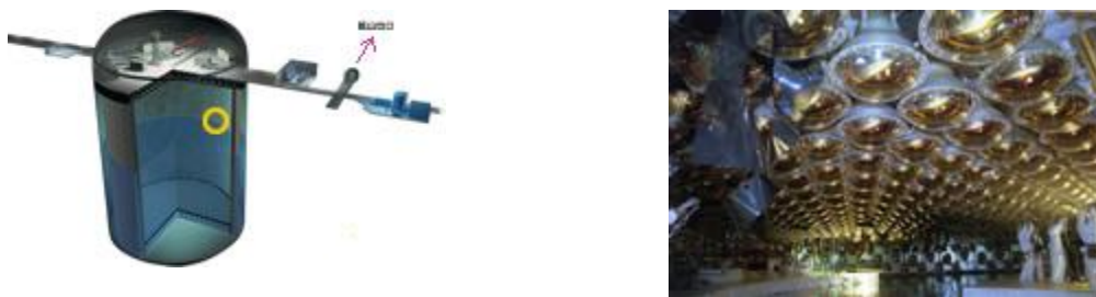
Fig4-3-5 Photo-Multiplier-Tubes (Inner detector)
