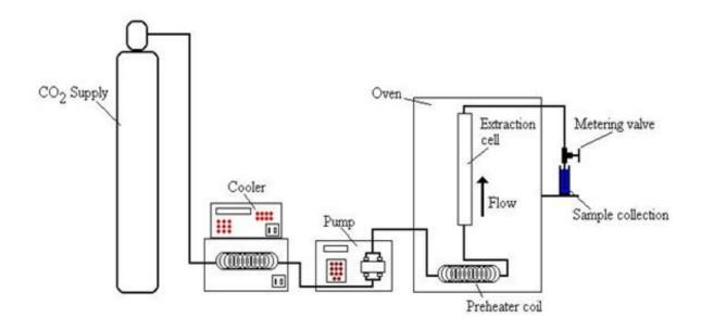
Extraction process is basically for separation of one component from other component by using extracting solvent. In SFE, we use supercritical fluid as extracting solvent with some co-solvent to increase its capacity to separate. For this type of extraction, we take sample of guava leaves 'mg in a cell column. In SFE CO' is mostly taken as super critical fluid with ethanol and methanol as co-solvent. Fig.' showing different components:
