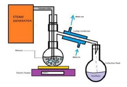
This process is basically for natural aromatic compounds used for temperature sensitive compounds which decompose at high temperature i.e.  $\Upsilon \circ$  mg of dried leaf material distilled in  $\Upsilon \cdot \cdot$  ml water. Process carried out for  $\Upsilon - \varepsilon$  hours at boiling temperature of solvent and after distillation, volatile compounds and water separated by methyl chlorate
