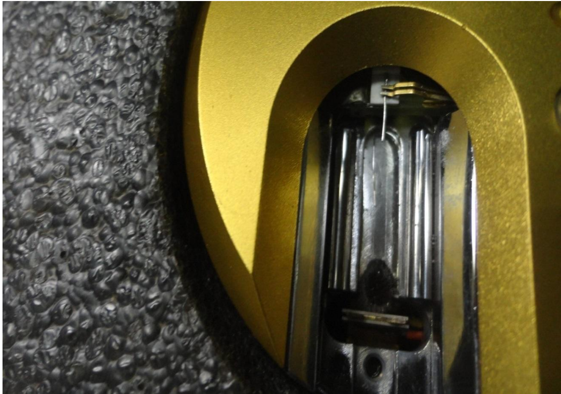
Figure (3.9): show a small sharp platinum tip used in easy Scan device
