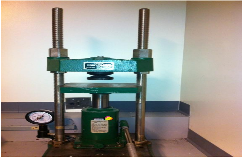
Figure (3.7): show compressive strength machine (Thomas, 2014)
