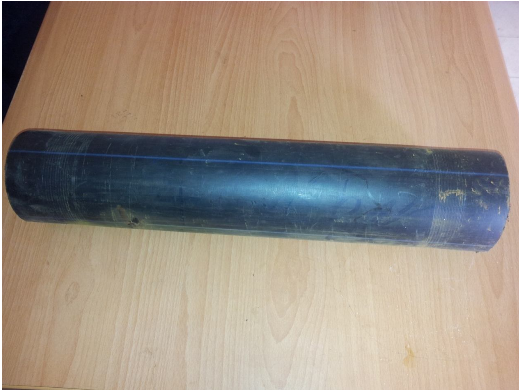
Figure: 3.1 sample of test High density polyethylene pipe.
