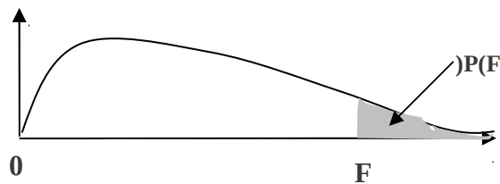
Fig(D.2)- F-distribution Curve
