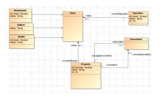
Figure 3.1 Class Specification Metamodel
