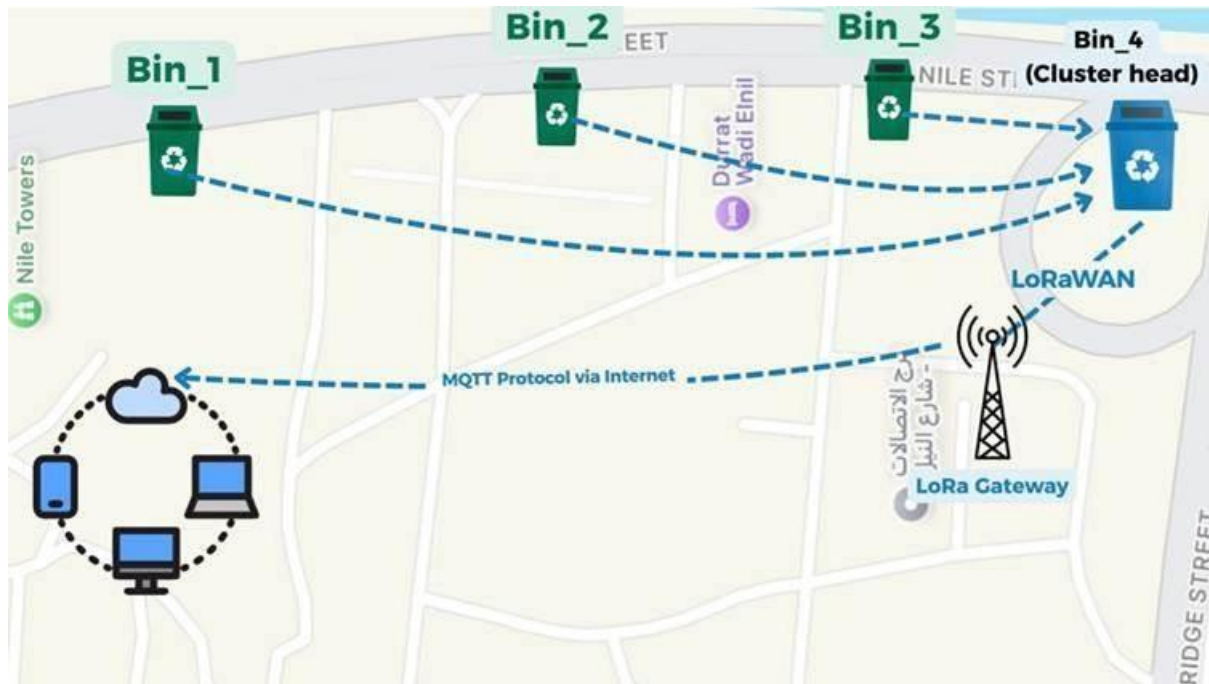
Figure 3.5: Layout of Clustered Smart Bins and Local Gateway Distribution along Nile Street.
