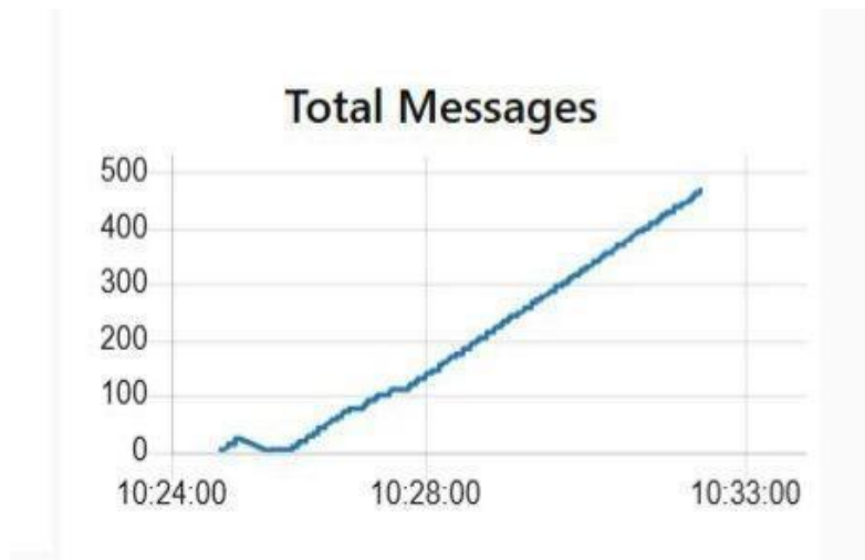
Figure 4.5.4: illustrate the messages interrupted when topic changed and restored when it retrieved.
