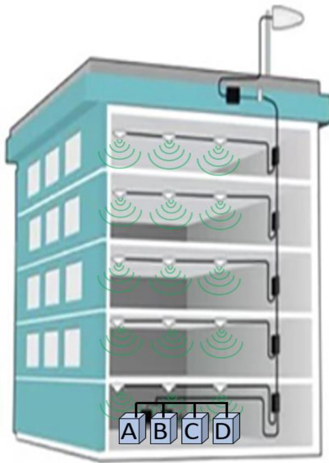
Figure 4.36. The shared IBS Indoor DAS site by 4 MNOs.
