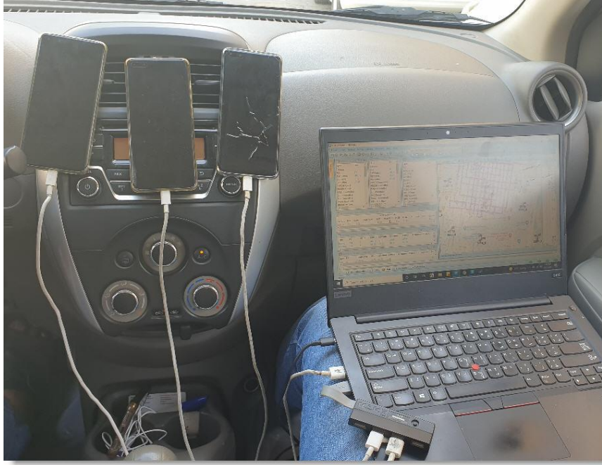
Figure 4.65. Photo of the car drive test tool used for field measurements.
