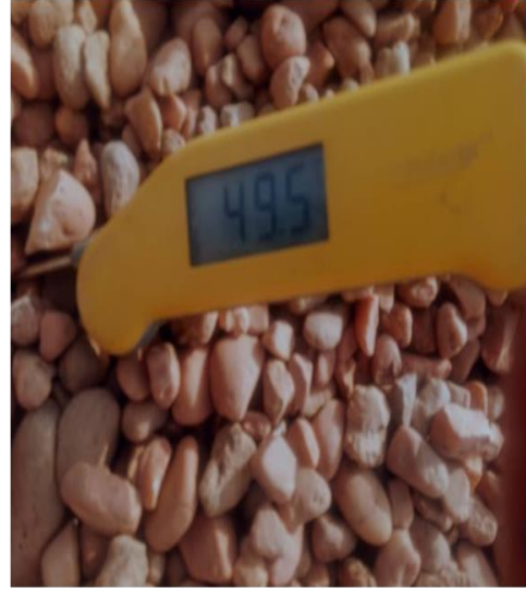
Heating the aggregate to a temperature 50 c°
