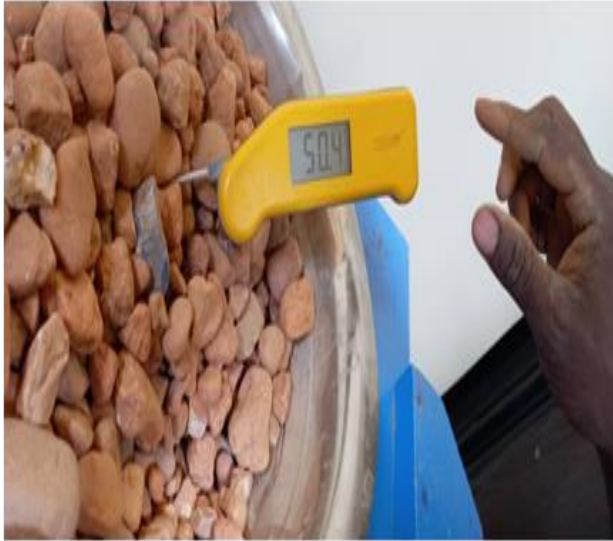
Heating the aggregate to a temperature 50 c°
