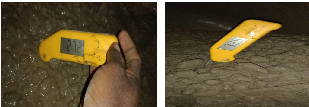
Figure4.12: Temperature of fresh concrete
