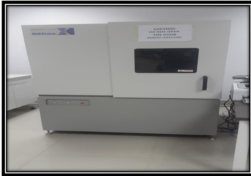
Fig (3.3) X-Ray diffract meter: XRD (wavelength 1.54 \text{ \AA} ),
