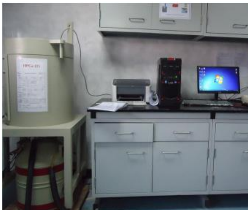
Figure 3.4: Gamma ray spectroscopy system with high purity germanium detector (HPGe )
