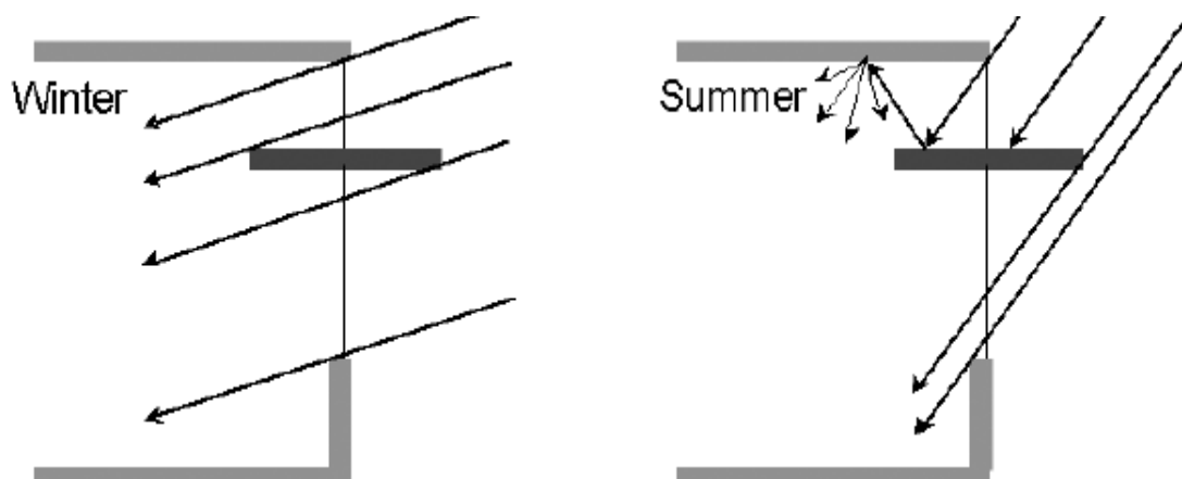
Figure 2-24 Sun ray guided by light shelf in winter and summer time Source: (Ruck et al. , 2000)
