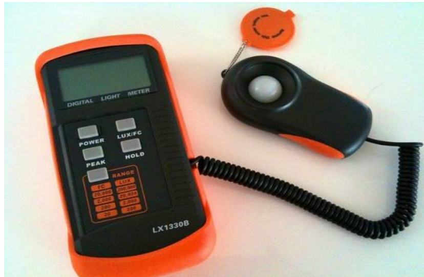
fig 4-10 daylight level measurement tool (luxmeter)
