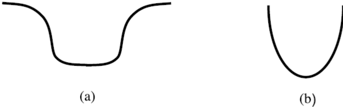
Fig 2.2 the mean potential and its approximation by a harmonic potential.
