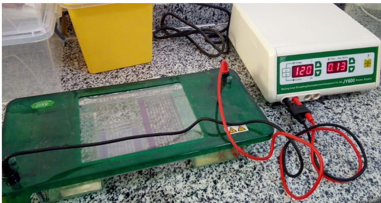
Color plate (4) :The gel electrophoresis apparatus was connected to the power supply (JY600; Beijing Junji-Dongfang, China)
