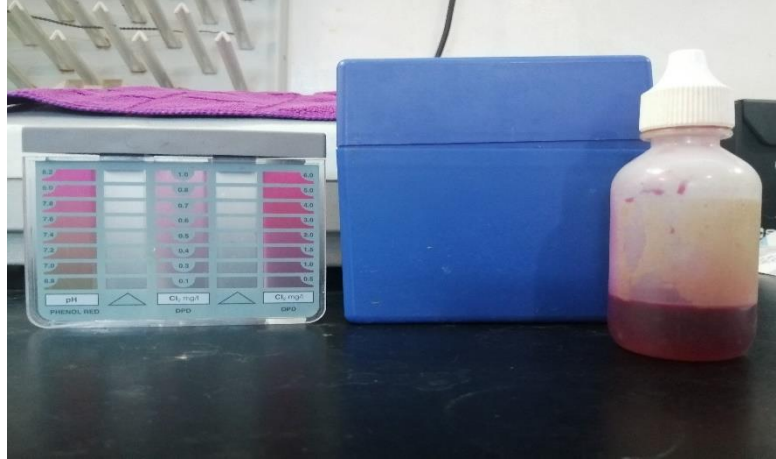
Figure (3-1): Colour Comparator Device, Phenol Red Index
