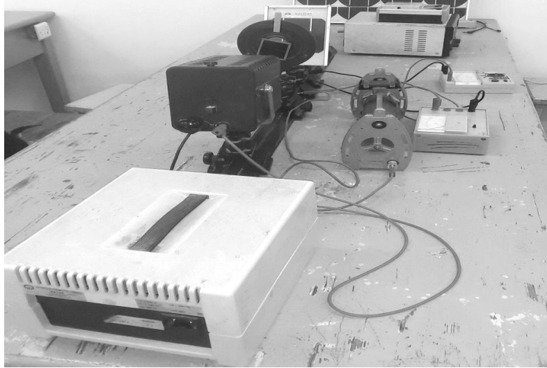
Figure 3.1 Experimental Setup for Recording the Current-Voltage Characteristics of a Solar Battery as Functions of the Irradiance
