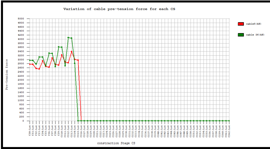
Figure (5-43): variation of cable pretension from cable 5 and cable 36 for each BCS
