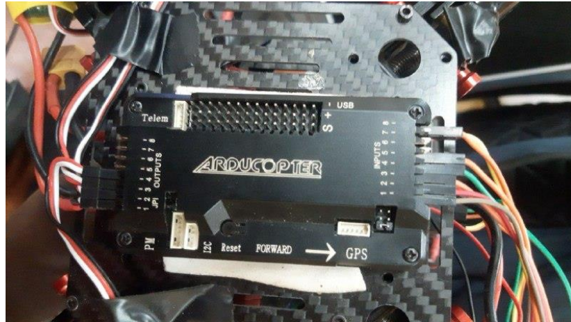
Figure 3-17: ESCs connection to Ardupilot Output and Receiver Channel Input
