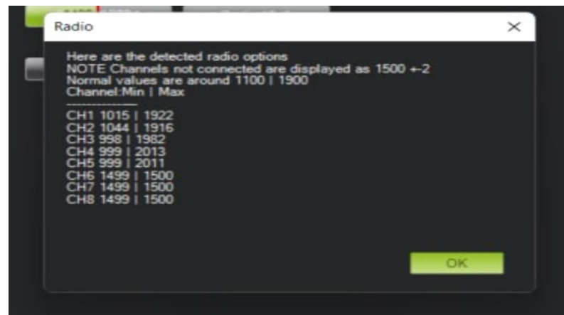
Figure 3-21: Transmitter Calibration Data
