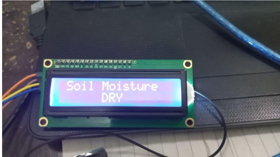
Figure 4-9: Soil moisture sensor status in the second case
