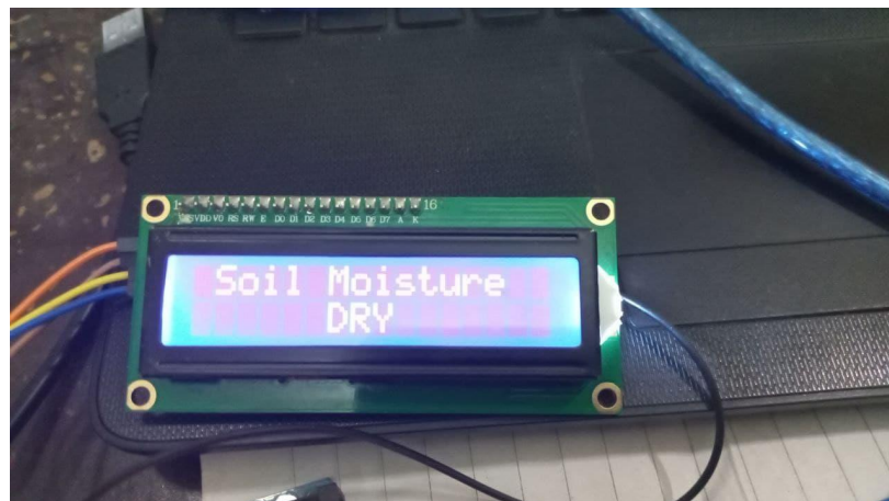
Figure 4-5: Soil moisture sensor status in the first case
