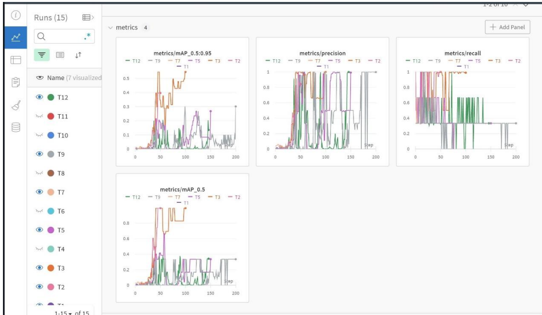
Figure 4-4: Plots of the precision, recall, Mean Average Precision (mAP) -0.5- parameters along with class object loss for training epochs
