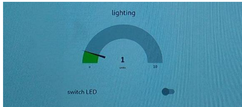
Figure 4-2: Screen shot of Light Dependent Resistor (LDR) readings on Node-Red dashboard
