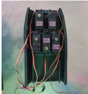
Figure 3. 10: ATTACHING SERVO MOTORS AT THE FOREARM
