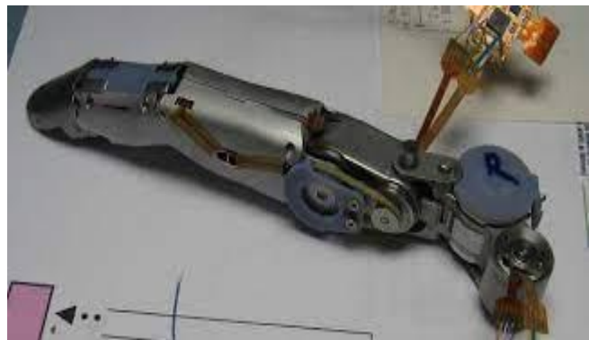
Figure 2. 12 22 Degree of Freedom APL Finger
