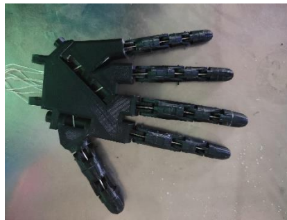
Figure 3. 9: SPREADING TENDONS THROUGH FINGERS
