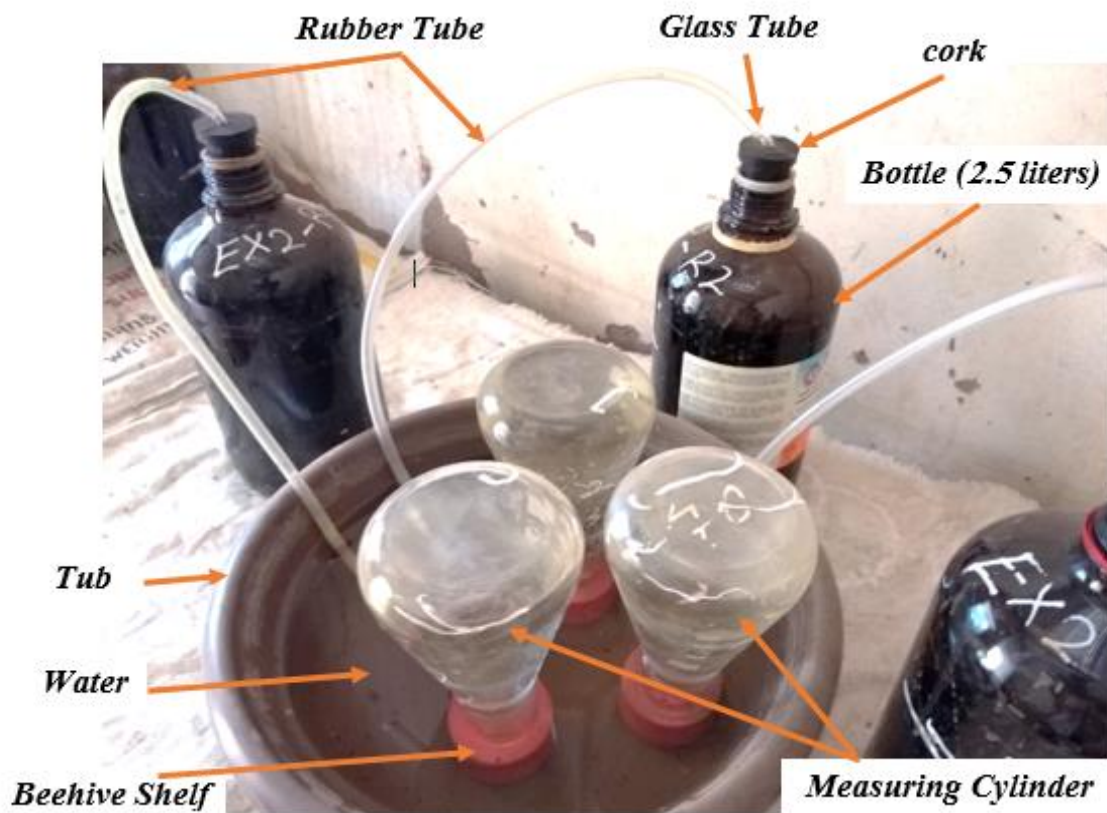
Fig (3.1.B): The Lab Scale of Anaerobic Digester
