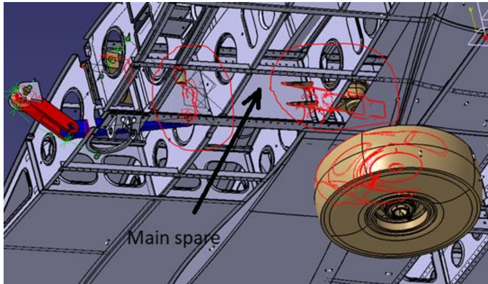
Figure 5.3: strut interference with wing main spar
