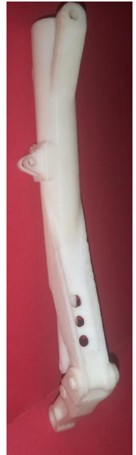
MLG manufactured by 3Dprinter
