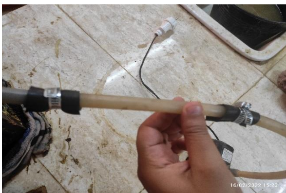
Figure 27 valves in the injection plastic hose
