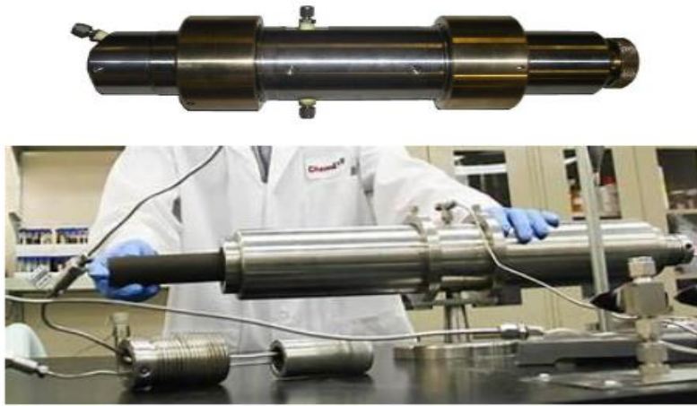
Figure 6 1D core flood model: used for linear flow.
