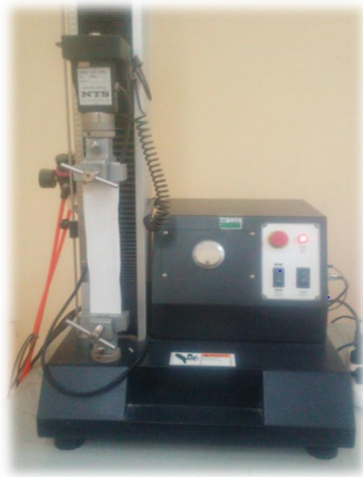
Figure 5-4: fabric tensile strength testing method
