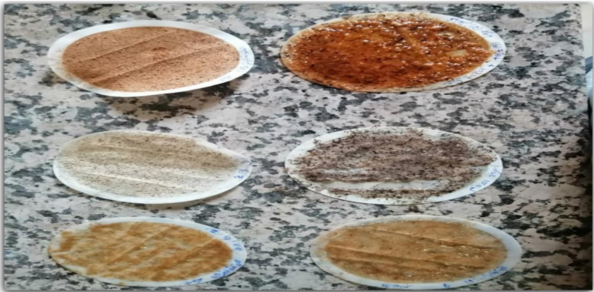
Figure (4.1) : filter cake for the local fluid filtration control materials
