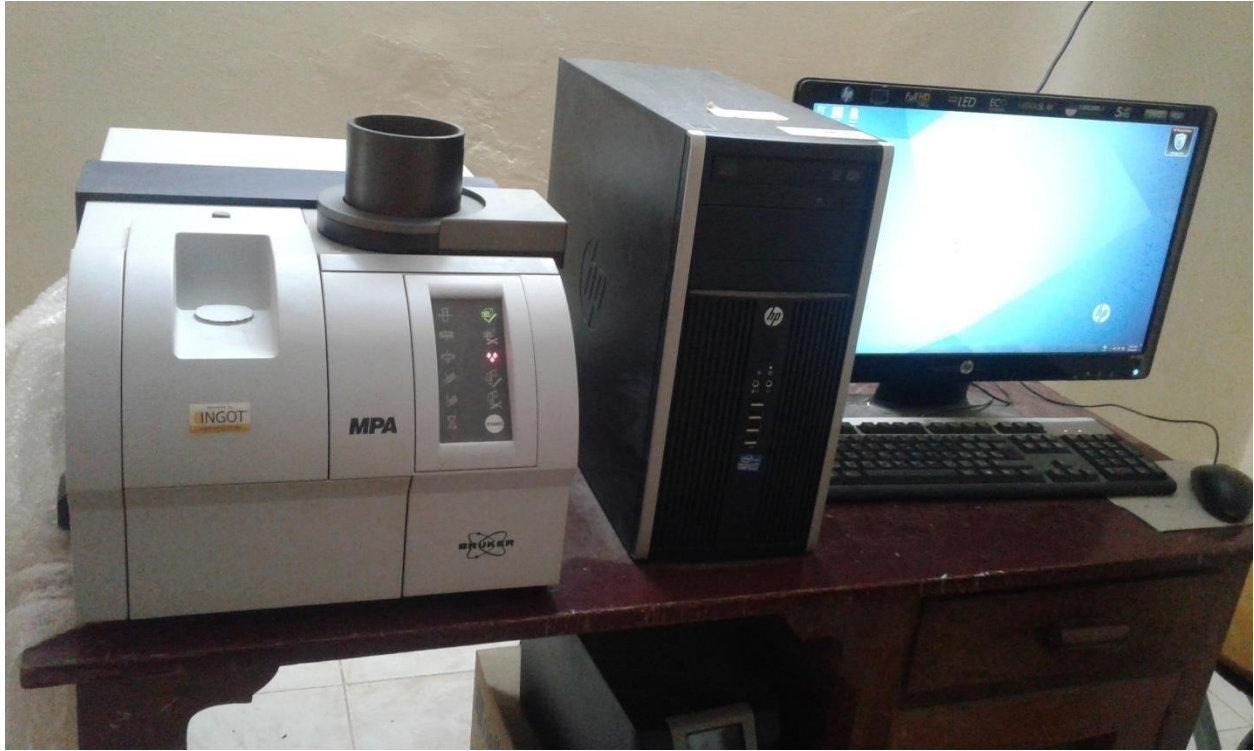
Appendix (9): NIRs, used in chemical analysis of fodder
