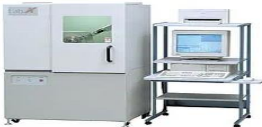
Figure (3.7): X-Ray Diffract meter: XRD (Wavelength 1.54\text{\AA} )
