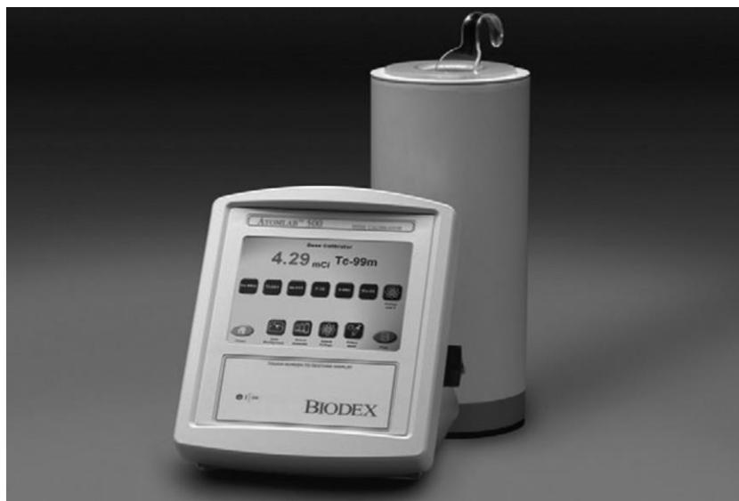
FIGURE 2.5 An ionization chamber dose calibrator. Samples are inserted into the well in the sealed ionization chamber. The current is measured and displayed on a digital readout. (Courtesy Biodex Medical Systems, Shirley, NY. )
